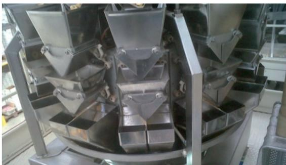
*The MF 52C model complete with a Multihead Electronic Weigher is a vertical packaging machine designed for various types of products with particular characteristics in terms of fragility, transferability, and grain size (pet food, pasta products, baked goods, snacks, vegetables, fourth range products, etc.).*
