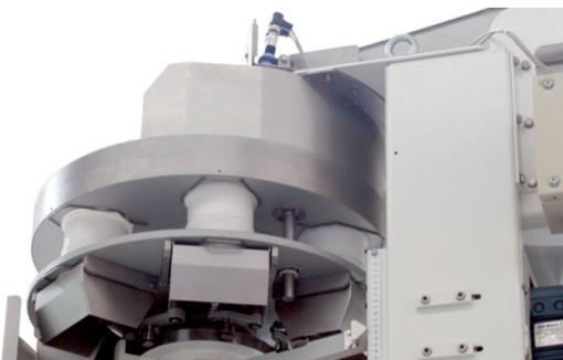
*As an alternative to the weighing system with multi-head weigher, the MF 52 C can be equipped with Cups Volumetric Rotary Dosing System, single or double.*
