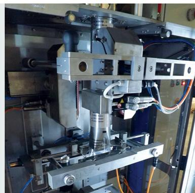
*Continuous vertical heat-sealing device with rotation controlled by brushless servo-motor, with constant temperature controlled by PLC.*
